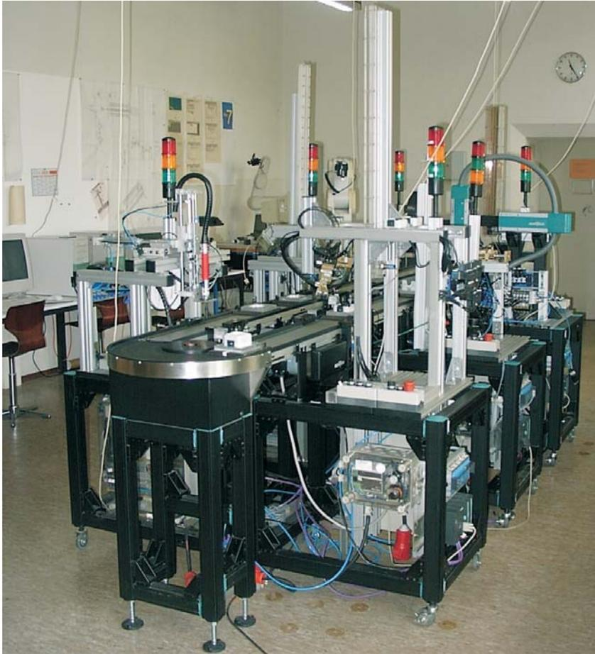
In the centre of the described vocational training stands an assembly line. Here electrical switches are mounted sequentially through a series of five assembly stations. Having reached the end of the assembly line the mounted switches are taken off it by a robot who puts them into boxes.
