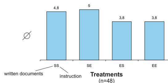
The main part of task 2 was to program the stations as far as possible. The diagram shows the average number of steps that were programmed by the four groups. According to the analysed data the students with the systematic oriented variant of the written documents in average programmed one step more than the groups with the example based material.
